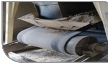
Fig.12 Unguarded material transfer point
