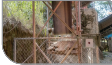
Fig.15 Gravity with emergency stop switch and fencing
