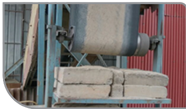
Fig.13 Unguarded gravity point in the conveyors
