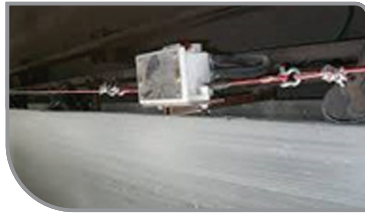
Fig.14 Pull cord and emergency stop switch
